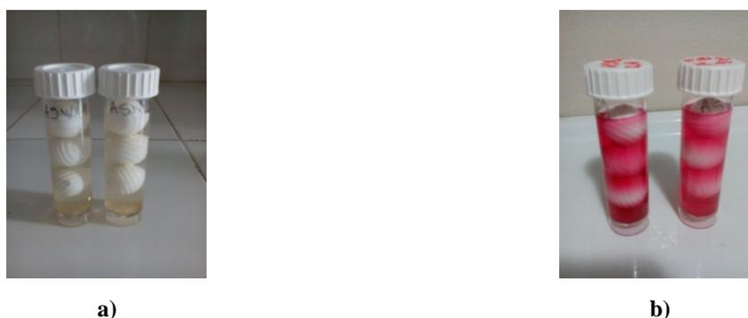
**Figure 4. Image of the results of N-Bart test for: a) initial filter backwashing water;
