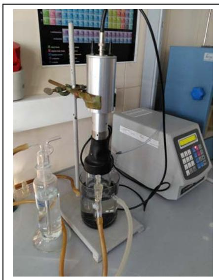
Figure 1. Ultrasonic reactor - closed system
