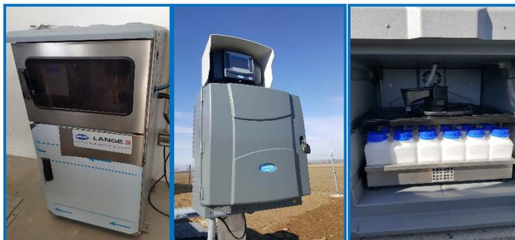
**Figure 2. Sampler for the daily and hourly collecting of the influent and effluent**
